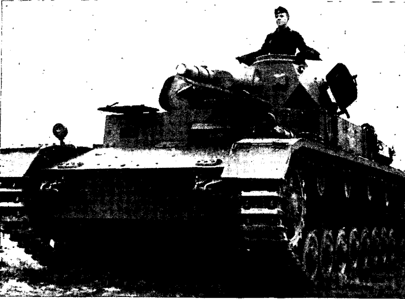
Figure 93.— Pz.Kw. IV (Sd.Kfz. 161) , medium tank, with short-barreled 75-mm gun.
