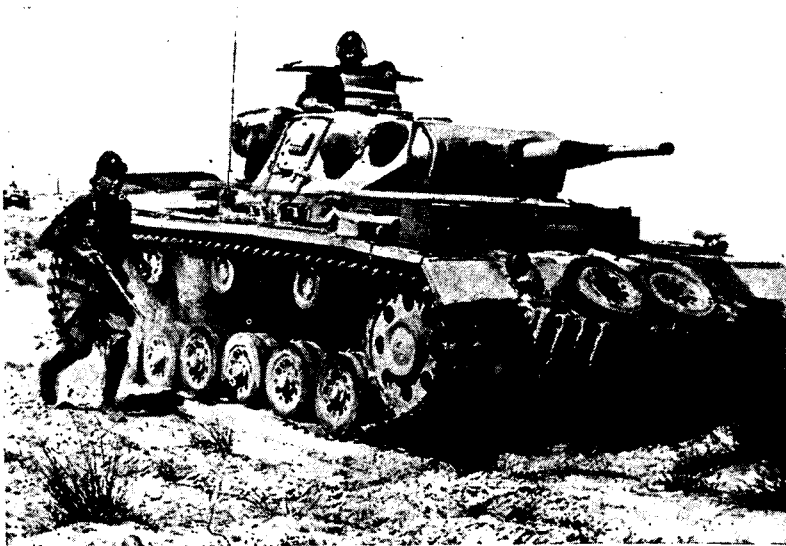
Figure 91.— Pz.Kw. III (Sd.Kfz. 141) , medium tank, with short-barreled 50-mm gun.
